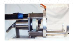
The **PROTEM SE219** has been especially designed and engineered to face and bevel tubes from 60.3 mm up to 219 mm OD. Its design and unique working range makes it the best tool in its class. The stainless steel or aluminium collet and its front support allow a perfect clamping and squareness with-out deformation for orbital welding. 4 standard HSS tool bits can be mounted on the tool holder plate to work simultaneously.
